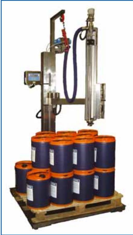
The **StrongArm** is a semi-automatic articulated arm filling machine which has been developed for the accurate filling of a wide range of industrial containers from 100 ml up to 1500 litres. This versatile machine can be configured to accommodate all aspects of filling including:
