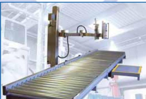
Our range of filling machines can be supplied as fully integrated systems to provide optimum operational efficiency. Options include complete motorised conveyor systems designed to synchronise the presentation of the empty containers to the filling head and then transport them away when filled. By taking responsibility for the complete system we can ensure everything works in harmony. Additional options include filling tables and a range of drum handling equipment.
